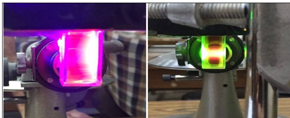
Fig. 12 The experimental fluorescence of new dye with pumping source 200 mw, 402 nm & 532 nm.
